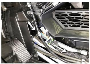
12. From interior of vehicle, continue routing harness through center console and out to engine area. Keep harness away from moving parts.
