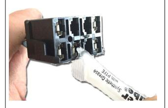
25. Connect switch to switch connector and install into dash, be sure to install switch into dash the correct way, RIGHT should be at top (side of switch is labeled).
