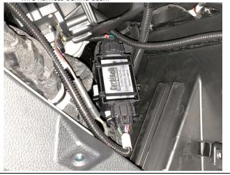
23. Determine location for turn signal control switch.
