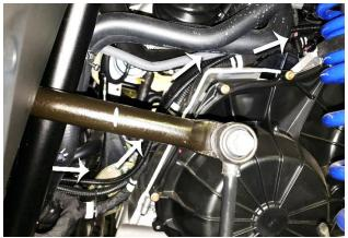
14. Locate wire connector and under driver side of cargo box frame. Unplug this connector and plug connectors B and C into the two available connectors.
