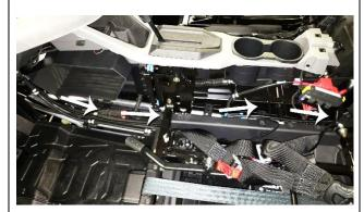
From driver side rear wheel area, continue routing turn signal harness toward rear of vehicle. Follow existing wire harness.
