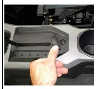
4. Remove plastic rivet and four bolts from driver side of center console.
