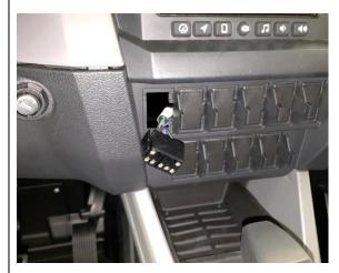
24. Apply dielectric grease to terminals on switch connector.
