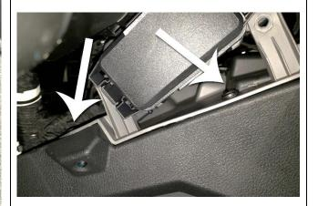
Remove side panel from center console. It will be difficult, start by sliding bottom away first while depressing gas pedal to get past it. Lift top of center console as needed to separate it from side panel. Make sure to unclip LED from side panel before completely removing panel from vehicle.
